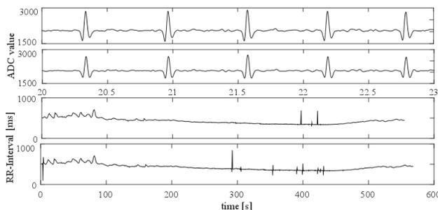
Figure 5. Results of treadmill exercise. Starting from the top: ECG (silicone electrodes); ECG (adhesive electrodes); RR-intervals (silicon electrodes); RR-intervals (adhesive Ag/AgCl electrodes)
