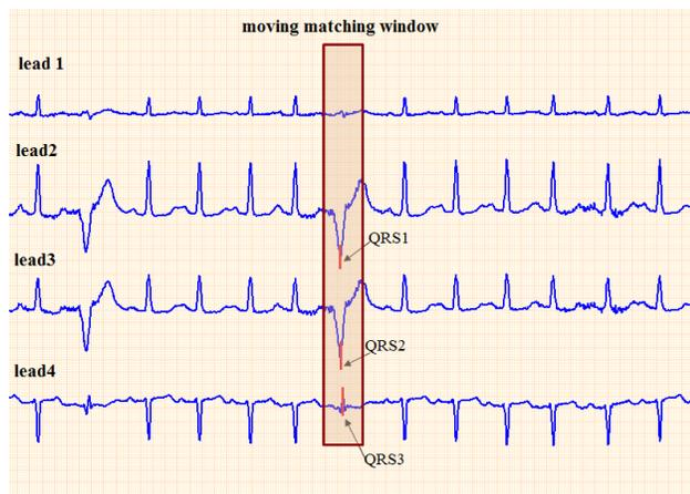
Figure 2. An example of four-lead QRS matching. QRS1, 2, 3 detected by single lead analysis are confirmed as a matched set.
