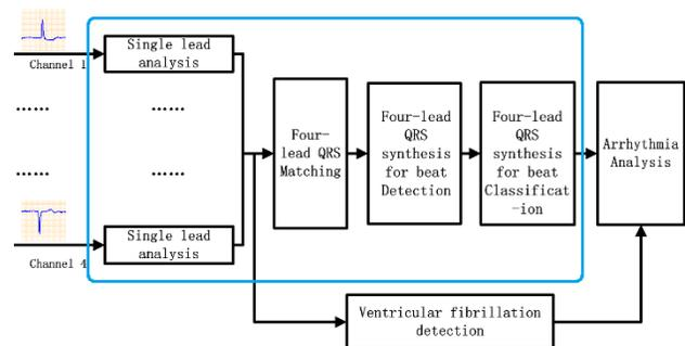
Figure 1. Schematic diagram of the four-lead real time arrhythmia analysis algorithm.
