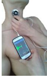
Figure 1. Acquisition of carotid audio signals using a stethoscope attached to a smartphone.
