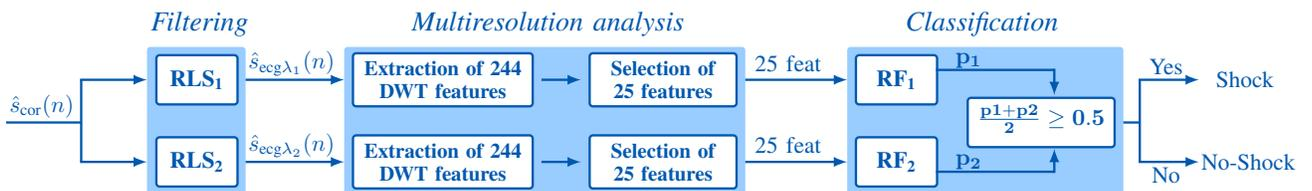
Figure 2. Architecture of the proposed double-stage SAA.
