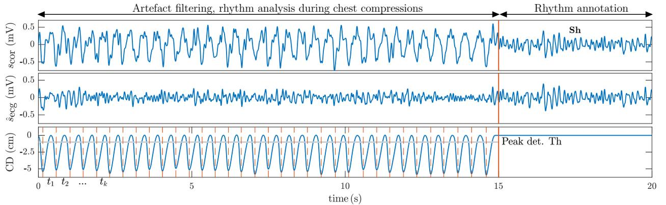
Figure 1. Example of a 20s episode of the database. The top panel shows the ECG of a patient with a shockable rhythm (Sh): the first 15 s are corrupted by the CC artifact and the last 5 s are free of artifact showing the patient's underlying rhythm. The second panel shows the filtered ECG and the bottom panel the CD signal with the CC instants ( $t_k$ ).
