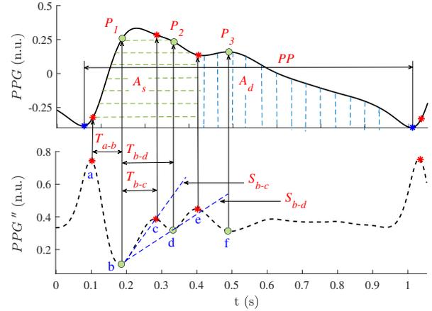
Figure 4. Detection of the amplitudes of a, b, c, d, e, and f waves of  $PPG'''(t)$  and estimation of pulse wave features of PPG;  $P_1$  - amplitude of the 1<sup>st</sup> systolic wave,  $P_2$  - amplitude of the 2<sup>nd</sup> systolic wave, and  $P_3$  - amplitude of the diastolic wave.
