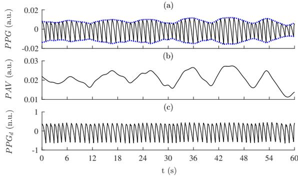
Figure 3. PPG amplitude demodulation during the *DB* stage: (a) PPG with the upper and lower envelopes; (b)  $PAV$  - difference between the upper and lower envelopes; (c)  $PPG_d$  - demodulated PPG signal.
