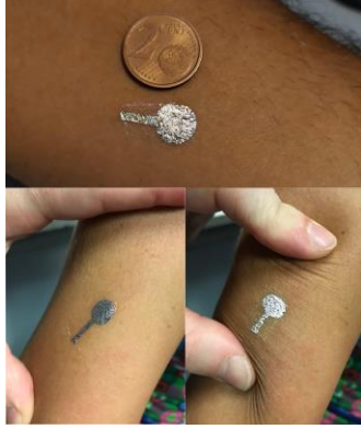
Figure 1. Examples of tattoo electrodes for ECG applied on the skin. As can be seen, they offer high skin conformability also when stretching or compressing the skin portion.
