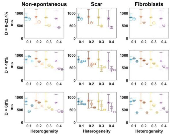
Figure 1. CLs of the tissue containing non-spontaneous cells, unexcitable cells and fibroblasts at different heterogeneities ( $\sigma$ ) and densities (D). Asterisks (\*) identify simulations with uncoupled cells, whereas circles (o) and squares (square) identify simulations with random and cluster distribution, respectively. Mean values  $\pm$  std.
