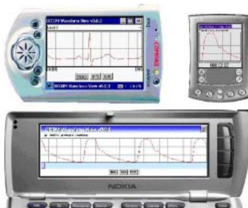
Figure 4. Mobile and PDA platforms capable of displaying DICOM waveforms including ECG files.
