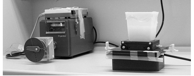
Figure 1. Image showing the phantom on the moving cart and the wire connection to the rotating disc. The angular velocity of the disc is controlled by a signal generator.
