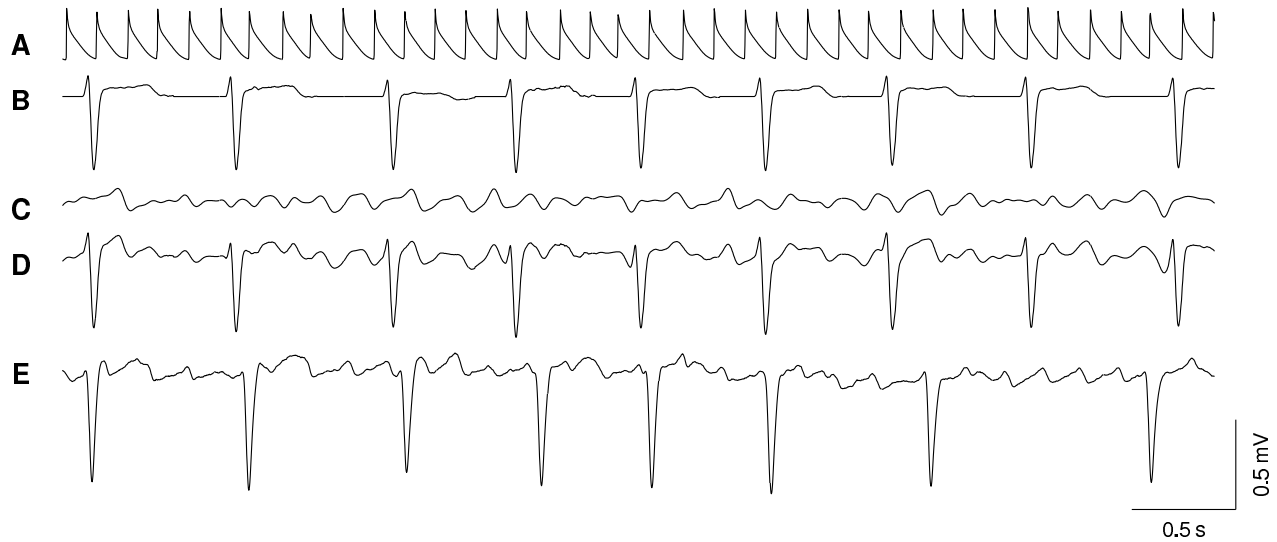
Figure 2. Construction of the synthetic ECG (lead V1): (A) Transmembrane potential computed close to the AV node; (B) reconstructed ventricular activity; (C) corresponding simulated AF activity; (D) complete ECG, i.e. sum of signals B and C; (E) example of a clinical ECG (also lead V1) during AF.
